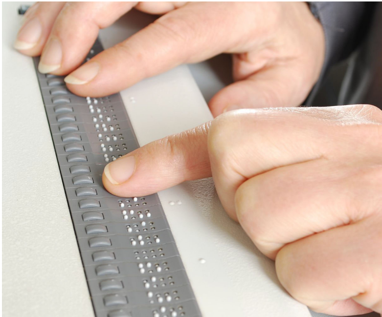
Fig. 10.1 A screen reader captures text on the screen and displays it on a Braille device
