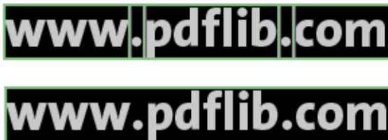
Fig. 6.5 The default setting punctuationbreaks=true separates the parts of URLs (top), while punctuationbreaks=false keeps the parts together (bottom).
